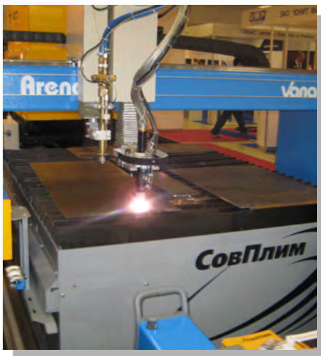
Sectional exhaust table CCT view 1
